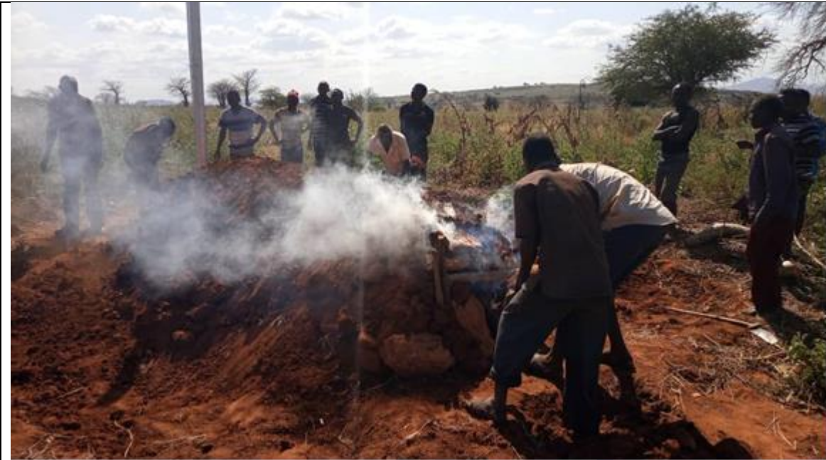
Practical training on how to start fire in the establishment of the Improved Basic Earth-mound Kiln (IBEK) at Kazania village.
