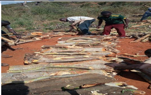
Charcoal producers at Kazania village placing railings and billets in the Improved Basic Earthmound Kiln.
