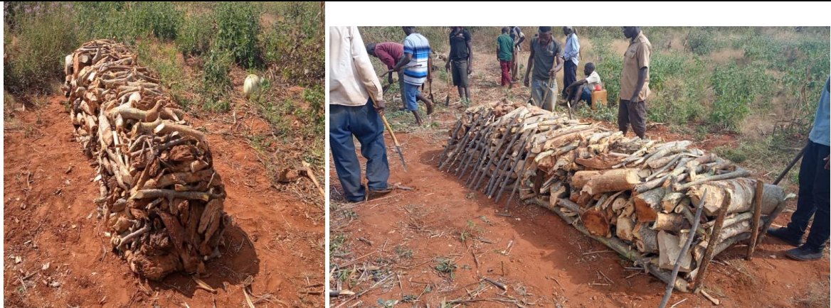
Charcoal producers from Kazania village placing apron sticks in an Improved Basic Earth mound Kiln
