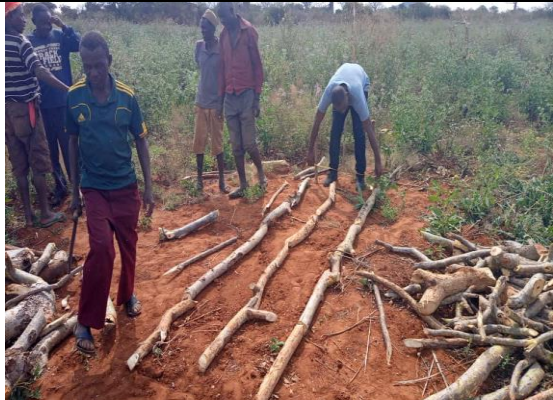
Charcoal producers at Kazania village placing railings and billets in the Improved Basic Earthmound Kiln.
